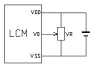
V<sub>DD~</sub>V<sub>0</sub>: LCD Driving voltage VR: 10k~20k
